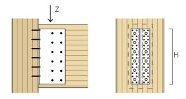
ALUMAXI with SBD dowels and LBA nails - partial nailing
