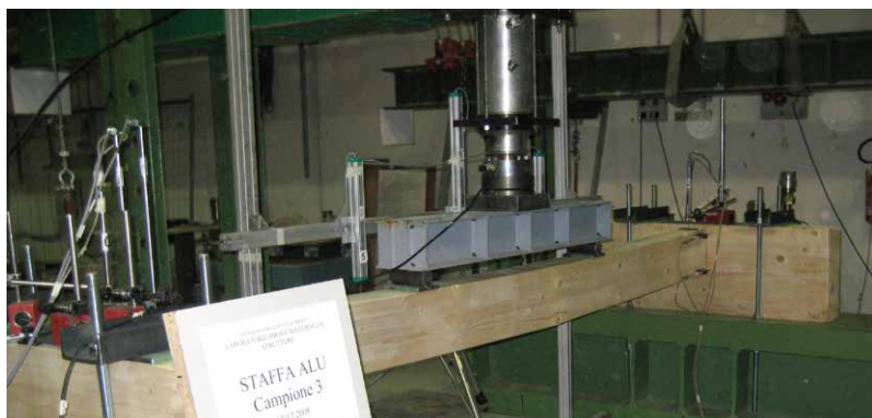
Tests on full-scale specimens (main-secondary beam connection).
